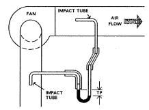
Figure D-7. Fan Total Pressure.
