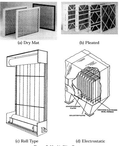
Figure D-29. Air Filter Types.
