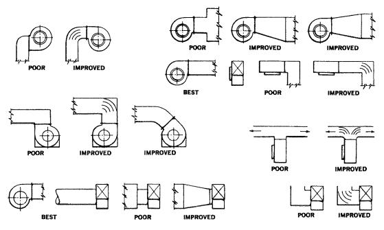
Figure D-26. Fan Outlet Conditions.
