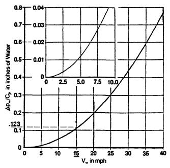
Figure D-3. Velocity Head vs. Wind Velocity.
