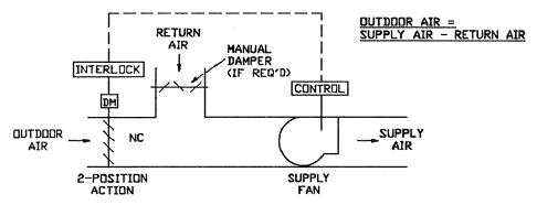
Figure D-41. Fixed Minimum Outdoor Air for Systems without Return Fans.
