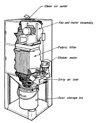
Figure D-32. Unit Collector.
