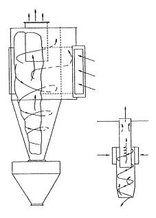
Figure D-36. High Efficiency Centrifugal Collector.
