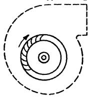
Figure D-14. Forward-Curved Fan.
