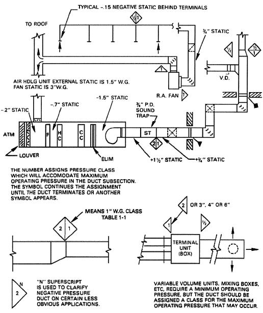
Figure D-28. Duct Pressure Class Designation.
