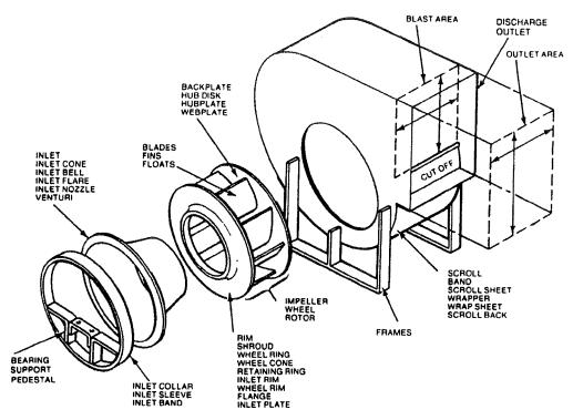
Figure D-10. Centrifugal Fan Components.
