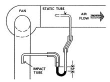
Figure D-6. Fan Static Pressure.
