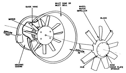
Figure D-15. Axial Fan Components.
