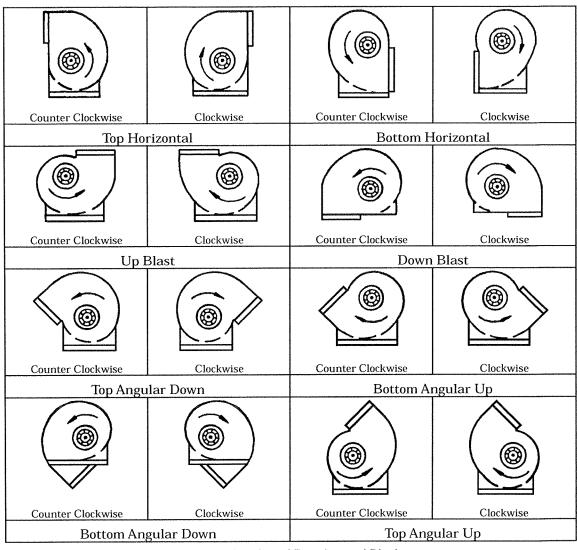
Figure D-25. Direction of Rotation and Discharge.
