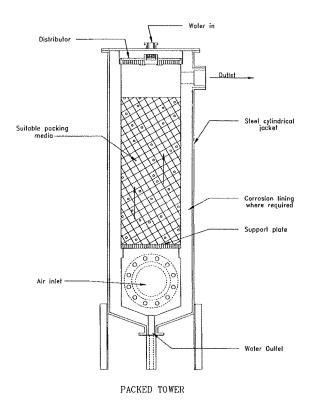
Figure D-33. Packed Tower Collector.
