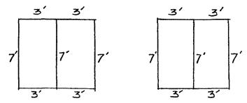
Figure D-2. Linear Feet of Crack of Windows.
