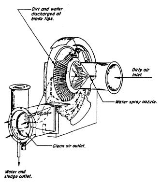
Figure D-35. Wet Dynamic Precipitator.
