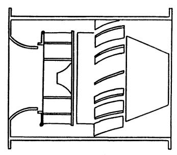
Figure D-19. Inline Flow Centrifugal Fan.
