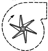
Figure D-13. Radial Blade Fan.
