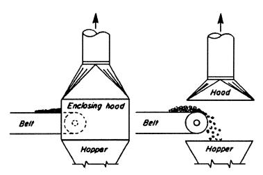
Figure D-38. Enclosed Hood (left) and Nonenclosed Hood (right).
