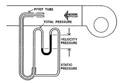
Figure D-8. Fan Velocity Pressure.
