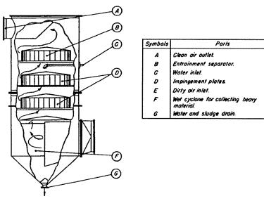
Figure D-34. Wet Centrifugal Collectors.
