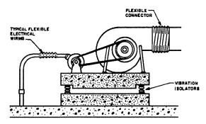
Figure D-27. Flexible Connections.
