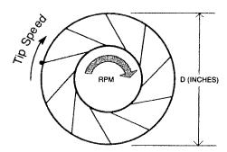
Figure D-9. Tip Speed.
