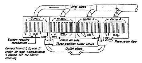
Figure D-31. Multiple-Section, Continuous-Duty, Automatic Fabric Collector.
