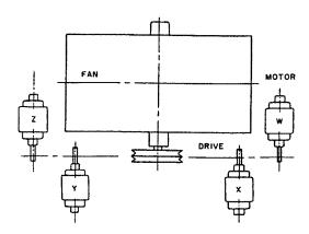
Figure D-24. Motor Positions.
