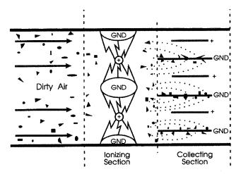
Figure D-30. Electrostatic Precipitator.
