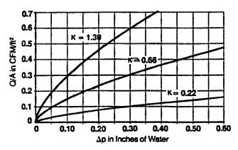
Figure D-4. Curtain Wall Infiltration for One Room or One Floor.
