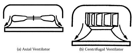
Figure D-20. Power Roof Ventilators.
